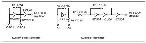
Figure 10 System Clock Oscillator and Subclock Input Specifications
